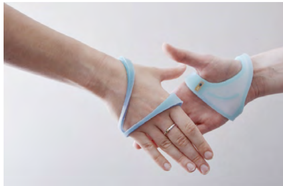
Fig. 5. and 6. (left) Meetspace in an inflated state. (right) Before the handshake, the wearables deflate each other to make room for the stranger's hand.
